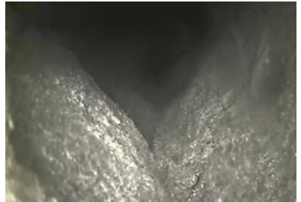
Water destroys the formation, washing it away during the traditional method of water at full pressure.
